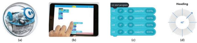
Figure 1. (a) The Sphero robot, (b) programming environment, (c) a sample program, and (d) interactive protractor for defining angles.
